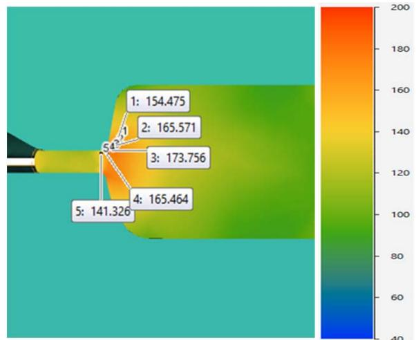
Fig.4 Field of effective stress at cross section near transfer radius of forging part
