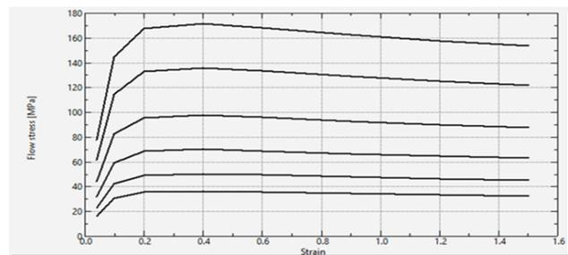
Fig.2 Flow stress for material S355J2 at temperature of 1100 °C
