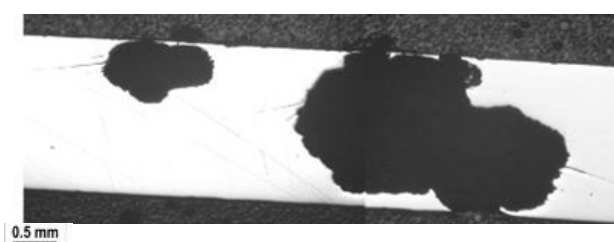
Fig.3 Cross section of the pipe in the corrosion zone
