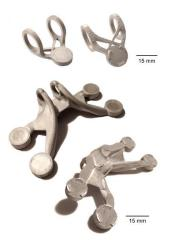
Fig. 2 Examples of parts made via ADAM in 17-4 PH [11]
