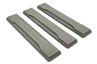
Fig. 3 Example of green parts printed via BMD in 17-4 PH stainless steel
